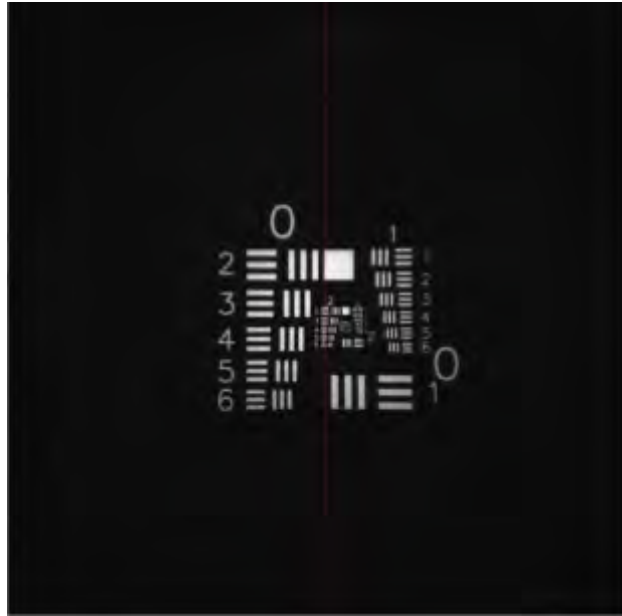
RMI context image. Similar to ChemCam w/ color. Spatial resolution of 65 \mu rad at -25°C (req. is 80 \mu rad)
